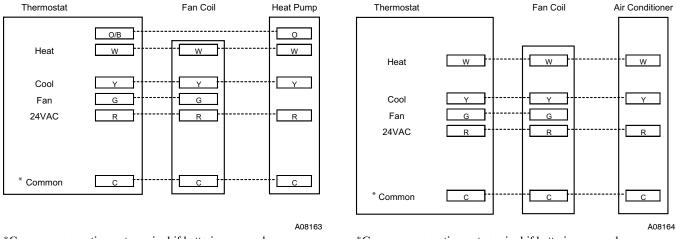
\*Common connection not required if batteries are used. Fig. 3 - HP Thermostat with Fan Coil \*Common connection not required if batteries are used. Fig. 4 - AC Thermostat with Fan Coil
